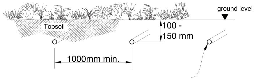
16 mm self-compensating drip irrigation pipe with emitters at 600 mm
