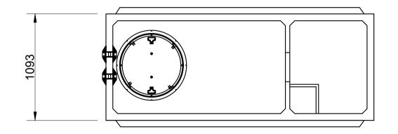
Lid thickness standard at 80mm. Recommended maximum loose soil cover depth - 400mm
