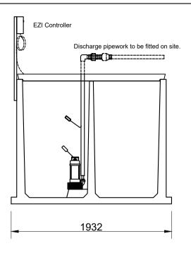
Unit supplied with 3 lift out concrete lids as standard. To extend with turrets use 400 dia Farm Tuff pipe.
