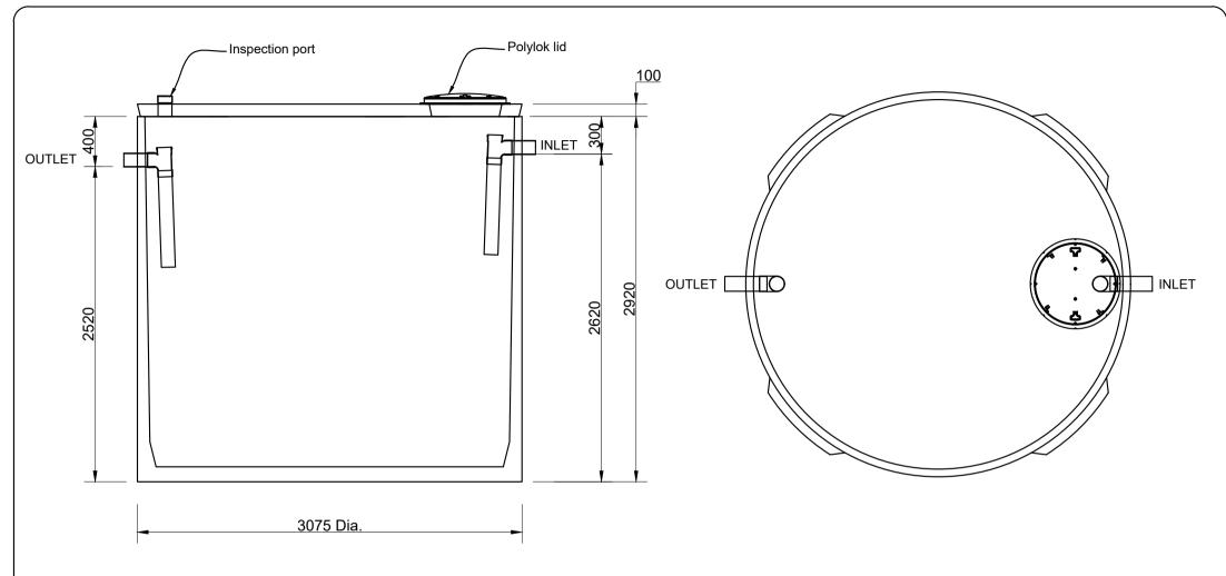
Unit supplied with Polylok lid as standard. 300mm riser increments available at additional cost if required.
