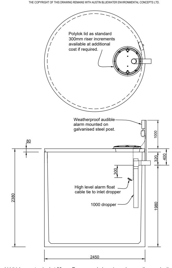
Lid thickness standard at 80mm. Recommended maximum loose soil cover depth - 400mm
