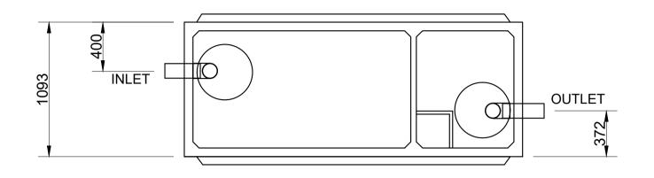
Unit supplied with lift out concrete lid as standard. To extend with turrets use 400 dia Farm Tuff pipe.
