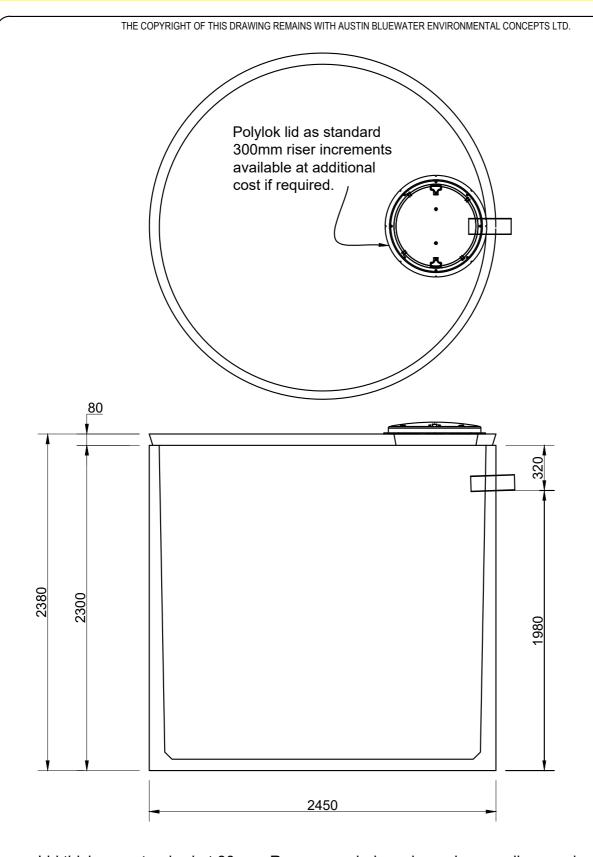
Lid thickness standard at 80mm. Recommended maximum loose soil cover depth - 400mm
