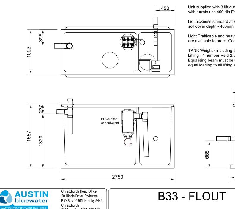
Unit supplied with 3 lift out concrete lids as standard. To extend with turrets use 400 dia Farm Tuff pipe
