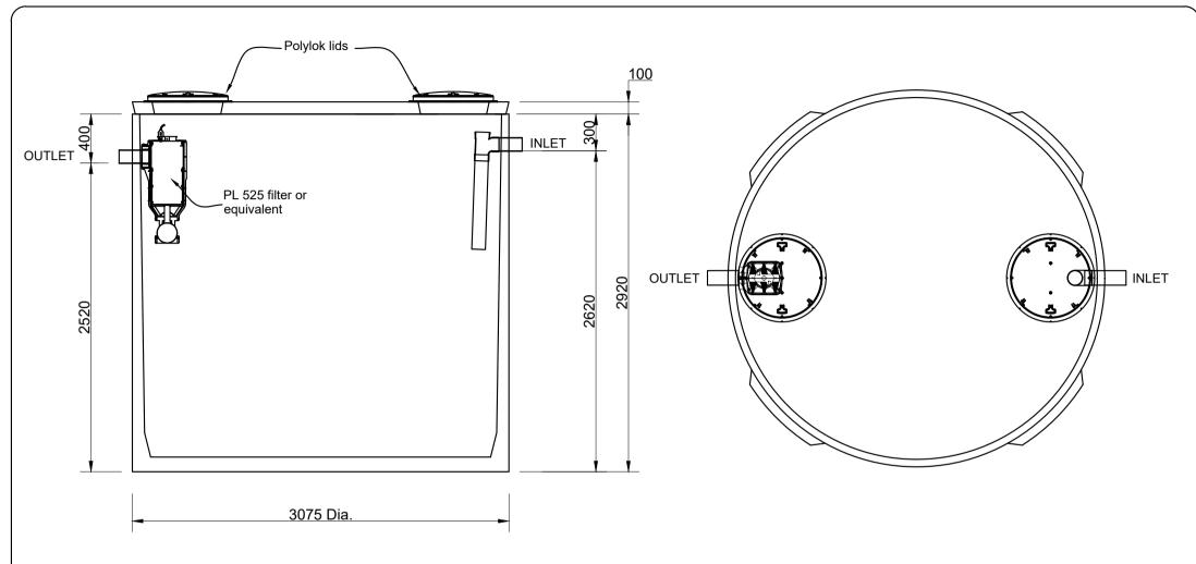
Unit supplied with 2 Polylok lids as standard. 300mm riser increments available at additional cost if required.
