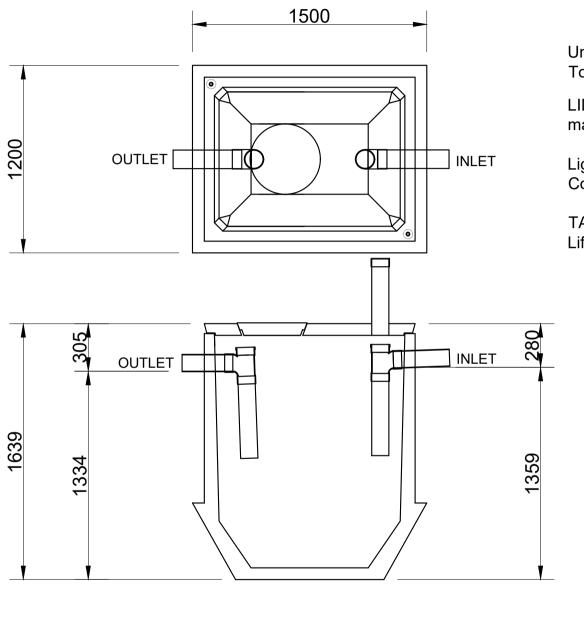
Unit supplied with lift out concrete lid as standard. To extend with turrets use 400 dia Farm Tuff pipe.
