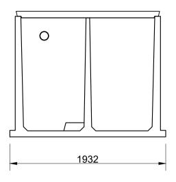
Unit supplied with 3 lift out concrete lids as standard. To extend with turrets use 400 dia Farm Tuff pipe.
