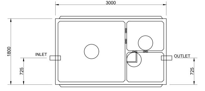
Unit supplied with 3 lift out concrete lids as standard. To extend with turrets use 400 dia Farm Tuff pipe.
