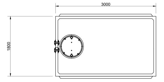
Unit supplied with Polylok lid as standard. 300mm riser increments available at additional cost if required.
