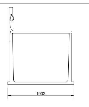
Unit supplied with Polylok lid as standard. 300mm riser increments available at additional cost if required.
