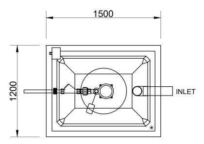
LID thickness standard at 80mm. Recommended maximum loose soil cover depth - 400mm.
