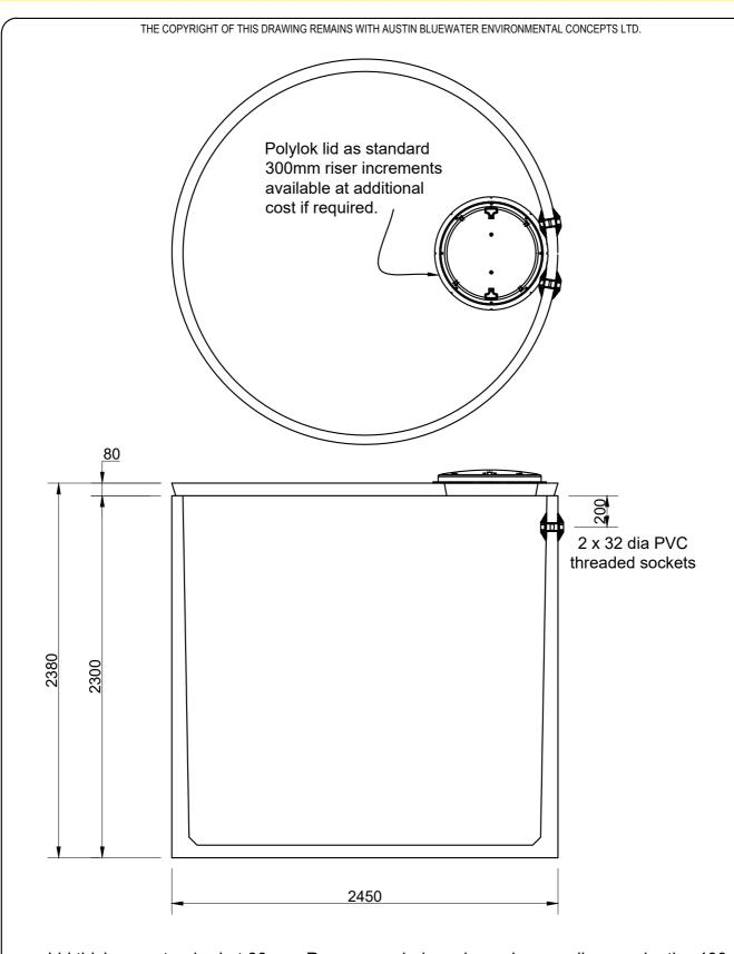
Lid thickness standard at 80mm. Recommended maximum loose soil cover depth - 400mm
