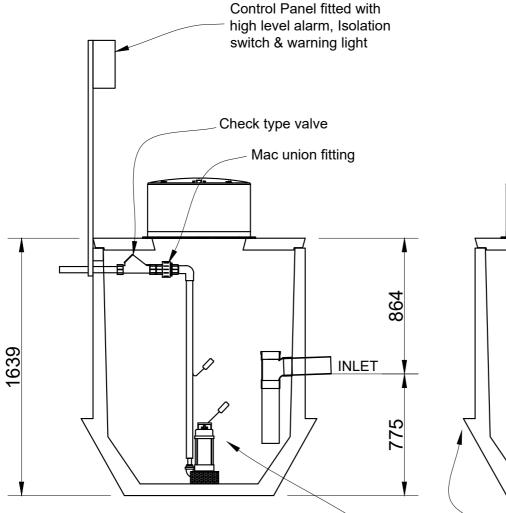
PUMP SYSTEM - Macerating, Vortex or Stormwater type pump, depending on application. Refer Technical Department for pump duty. 50 mm dia pressure pipe plumbing for Vortex or 32mm for Macerating.
