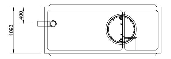
237 1557 1320 2750 Lid thickness standard at 80mm. Recommended maximum loose soil cover depth - 400mm
