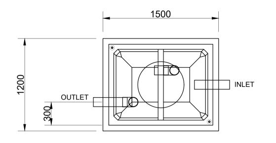
LID thickness standard at 80mm. Recommended maximum loose soil cover depth - 400mm.
